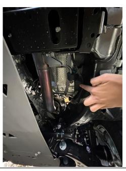
**Step 6 Toggle Only:** Route the battery terminals of the Off/On Harness (64-0139) back to the battery along the general path depicted below. Take care to ensure the harness avoids all hot, sharp and rotating components.
