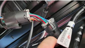
**Step 5 Toggle Only:** Attach the 10 foot extension (64-0165) to the 55" splitter as shown in the picture. Route this harness all the way up to the front of the vehicle. The extension will be used to connect this harness to the main On/Off harness (64-0139) coming at the front of the vehicle. Follow preexisting wiring and brake lines where possible.
