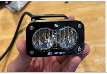
**Step 2:** Find the location shown in the picture below for mounting the lights. Take out the OEM bolt from the vehicle's rear bumper using a 10mm socket. Use the slot provided on the bracket to mount the light on the vehicle with the removed OEM bolt. Use 10mm wrench to tighten the bolt. Align the Reverse Bracket (44-7706) so make sure the light is pointing in the right direction.
