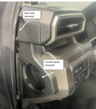
Remove the trim panel off the side of the dashboard by starting at the top edge and gently pulling away from the dash. Remove the chrome trim panel by pulling parallel to the arrows pictured.
