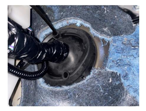
Pull the switch lead into the engine bay until it is long enough to be reconnected to the original harness. Re-install the white connector onto the exposed pins using the format below and then reconnect the two harnesses.
